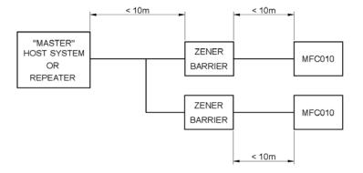
Each MFC010 <u>MUST</u> have its own dedicated barrier interface; they <u>MUST NOT</u> be connected in parallel on the hazardous area side of the system.
