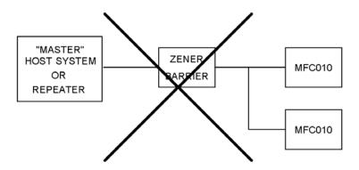
In a multidrop installation, see figure below, the Zener Barrier devices must be connected to the bus using a suitable RS485 repeater, with the connecting cable between the Barrier devices and the repeater not exceeding 10 m. The connection of the repeater to the Modbus busmust then follow the rules and restrictions of the Modbus protocol as indicated previously in section 3.4.
