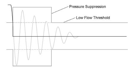
The amplitude, frequency and decay rate of the ringing effect will depend upon the flow rate prior to the Flow "Switch Off", the rate at which the "Switch Off" occurs and the damping characteristics of the pipe work i nstallation. F or this reason, setting the parameters of the P ressure S uppression function is an empirical process that the installer must go through to optimise the operation to the target installation.
