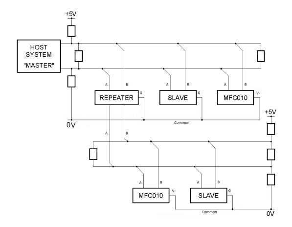
**NOTE** For Hazardous Area applications the user should refer to section 4.3, on page 21, for connection details.
