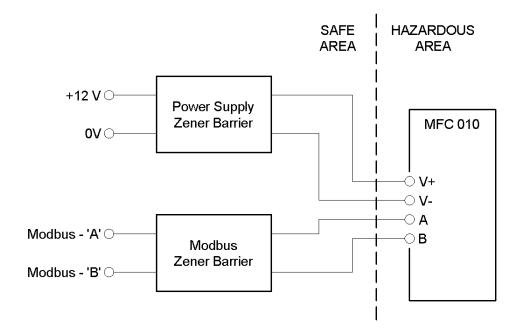
Inside the safe area, make a branch connection (2 wires plus "Common") from the main bus i nto a separate el ectrical c abinet w here s upply v oltage ( nominal 100... 230VAC, 50... 60Hz, or 24V DC) i s available.
