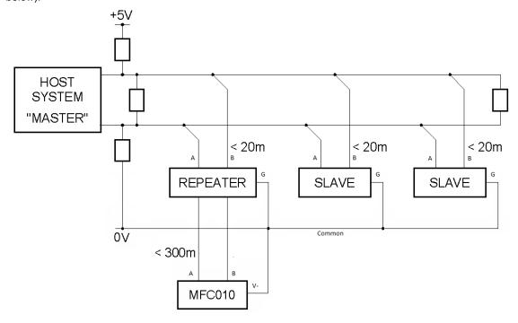
Because the connection to the bus requires exposing the signal wires, the connection to the main bus must reside in housing:
